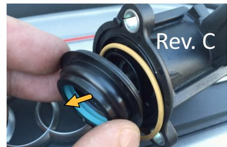
Install the GFB parts onto the solenoid body as shown below, using a little engine oil on the outside of the piston. **Make sure to use the GFB supplied spring inside the solenoid coil** – the only factory parts you re-use are the solenoid coil and the yellow o-ring.
