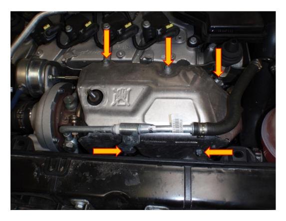
2. With the original heat guard left in place fit the Forge blanket over the top of it. Line up the holes at the top first and using the supplied 3x M6 fasteners and penny washers secure to top half of the blanket, do not fully tighten at this stage.
