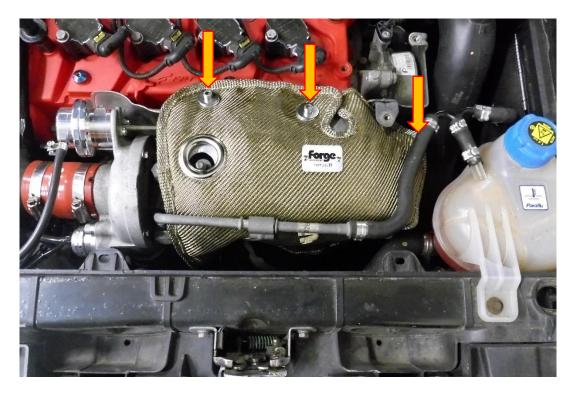
3. Stretch the blanket over the threaded studs and secure into place with the two supplied M6 nuts.
