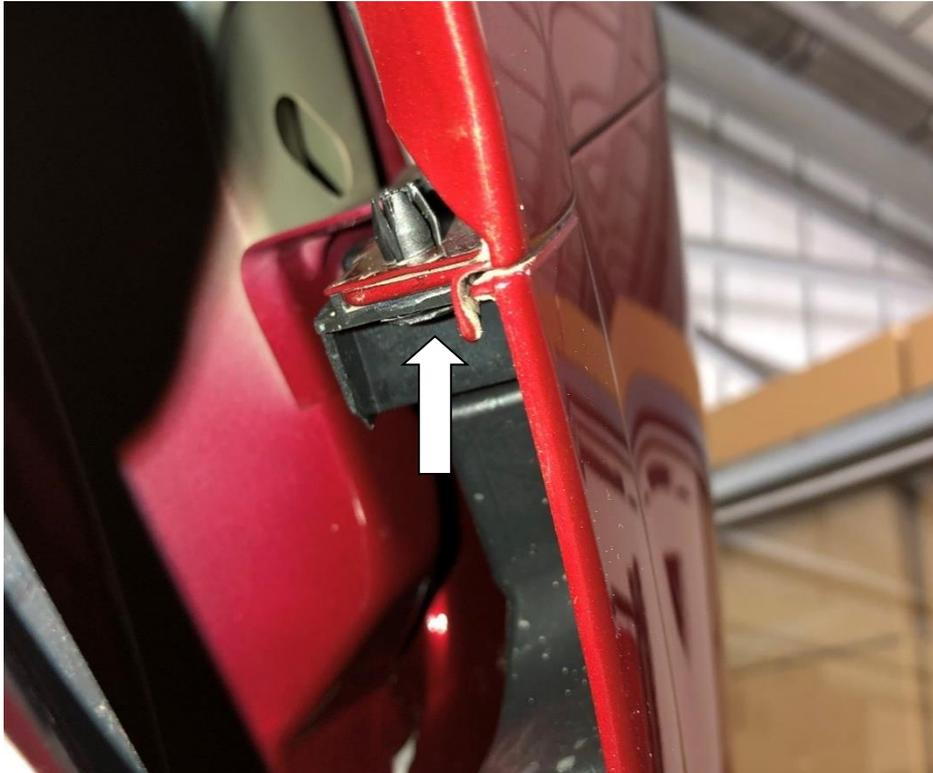
9. Carefully pull the edge of the bumper away from the vehicle starting at each wheel arch.
