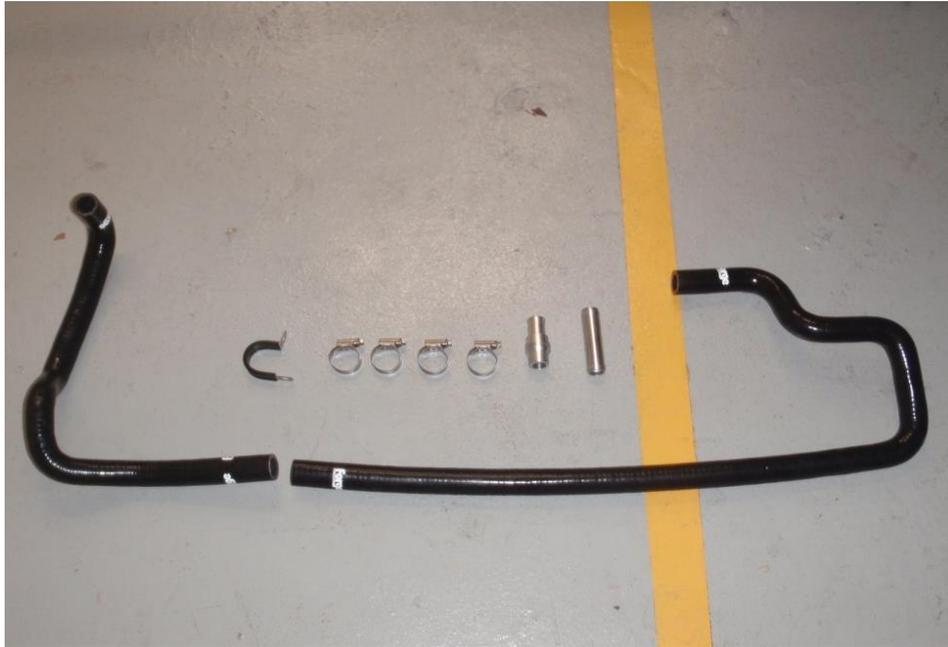
24. Fit the coolant coupler to the hose (marked #1888) provided as shown in the photo below and secure the coupler with a suitable hose clamp provided.
